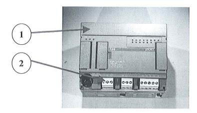
Open the product to separate in two parts: (lower part: power supply and I/O boards and the top part: UC board)
